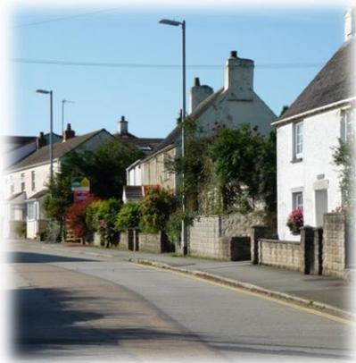
They have traditional dual pitched roofs; some properties to the rear have flat roofs. These consist of slate, fibre cement, asbestos and thatch. One of the properties also has dormer windows. The walls are a mixture of painted render, natural stone, brick and pebble dash. Some of the older properties are constructed of cob. Lanhadron is a thatched property and is the only listed property on the street scene.
