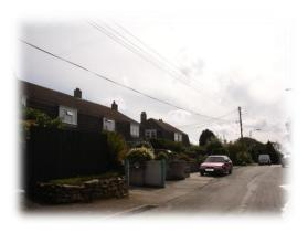
The roofs are concrete tiles with chimneys and the walls are pebble dash or brick with hanging concrete tiles. The windows and doors are uPVC glazed.
